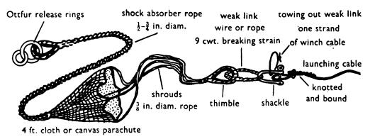
Fig. 4. The cable make-up.
