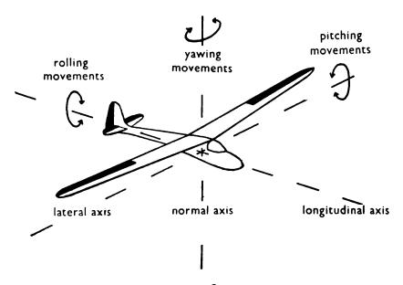
Fig. 6a. Axes of movement.
