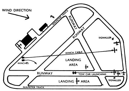
Fig. 2. The layout of an airfield gliding site.
