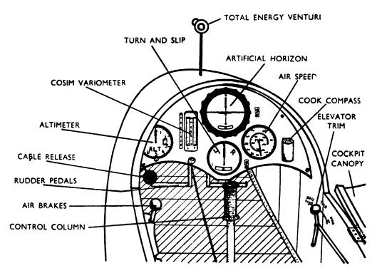
Fig. 3. The cockpit layout of a modern glider.
